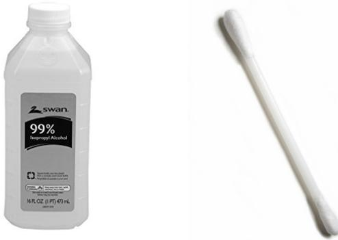
To clean, you dip your q-tip in the alcohol then vigorously scrub each metal element in the tape path. This includes: the tape guides, the tape arms, the tachometer, capstan, and of course the tape heads. Clean each element until nothing more will come up. For the tape heads, you want to scrub horizontally NOT vertically. You will use up many q-tips doing this.
